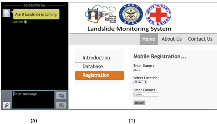
Figure 21.10 An SMS alert generated from the IoT landslide monitoring framework on a mobile phone. (a) The mobile interface showing the SMS alert. (b) The web-based interface for landslide monitoring.
