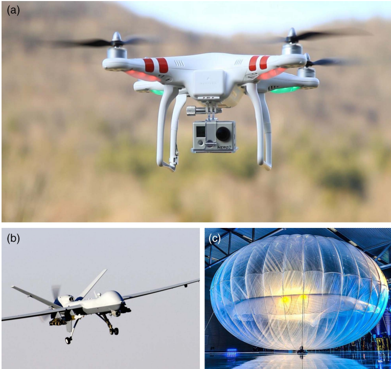
Figure 19.1 Examples of UAVs. (a) A drone. (b) A remotely piloted aircraft. (c) A balloon.
